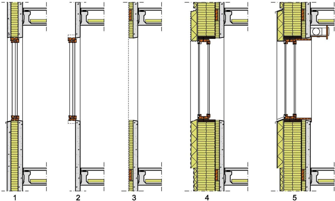
*Fig. 2 The outermost concrete layer of the sandwich element is dismantled (2) and the existing thermal insulation removed. 70 mm of thermal insulation is mounted on the concrete surface (3) to make the surface even enough for the elements. The facade element (4) has 350 / 400 mm of thermal insulation. The windows, the balcony doors and the vertical ductwork for the supply air are installed in the elements. The finishing work is done on site (5). Image: Kimmo Lylykangas Architects.*
